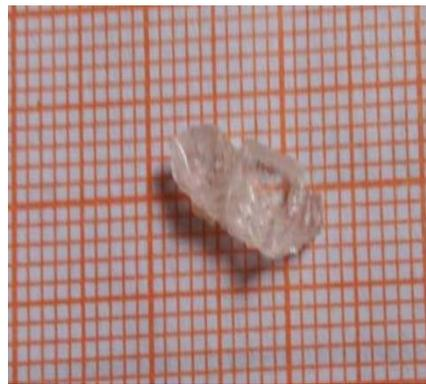
**Figure 7.** Show a picture of the glycine sodium nitrate crystal.
