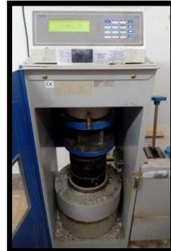
Fig. 7. Compression testing machine
