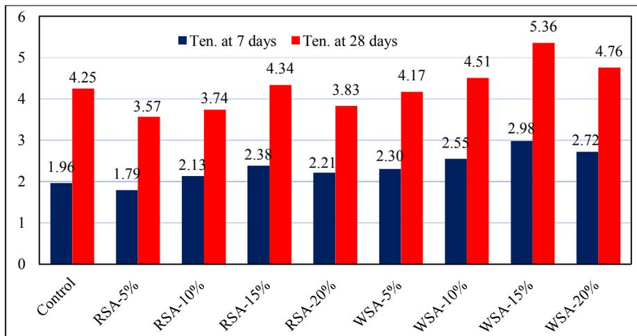
**Fig. 11. Tensile strength at 7 & 28 days**
