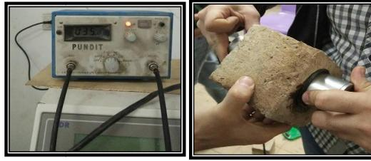
Fig. 9. Ultrasonic test
