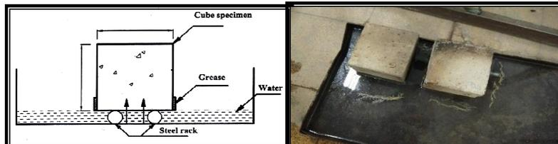
Fig. 10. Sorptivity test
