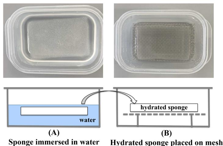
**Figure 1.** Experimental system for measuring weight change and water absorption and water retention of collagen sponge: (A) Sheet-shaped sponge was immersed in water for a predetermined time and then the weight of hydrated sponge was measured. This experiment was performed using 8 containers ( $n = 8$ ). (B) Hydrated sponge was placed on a 10-mesh size stainless steel mesh and weighed at predetermined time intervals. This experiment was performed using 8 containers.
