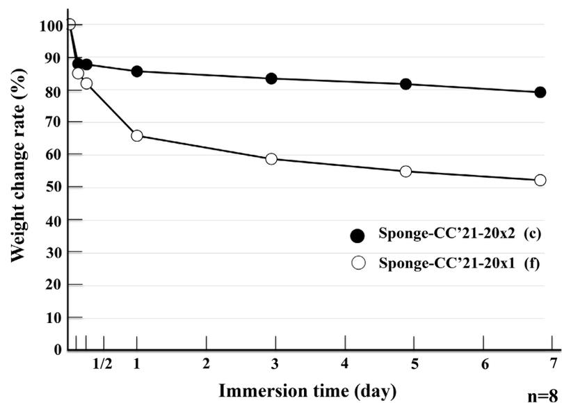
**Figure 4.** Weight change rate (%) of Sponge-CC'21 when immersed in water: (●) Sponge-CC'21-20x2 (c) (○) Sponge-CC'21-20x1 (f).
