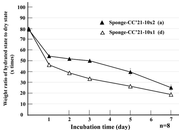
**Figure 6.** Weigh ratio of hydrated state to dry state of sponges (x times): (▲) Sponge-CC'21-10x2 (a); (△) Sponge-CC'21-10x1 (d).
