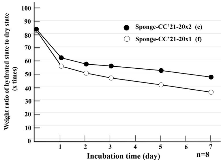
Figure 8. Weigh ratio of hydrated state to dry state of sponges (x times): (●) Sponge-CC'21-20x2; (c) (○) Sponge-CC'21-20x1 (f).
