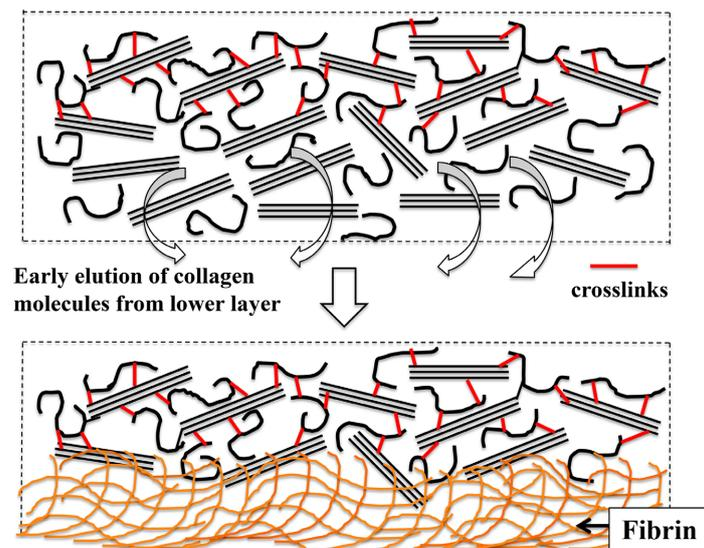
**Figure 11.** Schematic diagram of single-sided UV-irradiated sheet-shaped sponge: non-cross-linked collagen molecules in the lower layer elute first, and then the fibrin network structure is formed.
