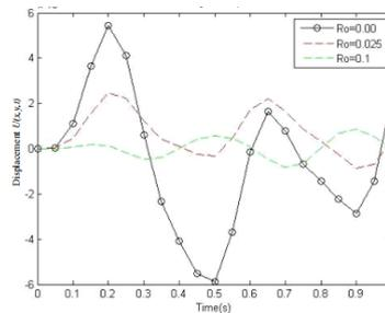
Figure 2. Effect of Rotary Inertia on Moving Mass
