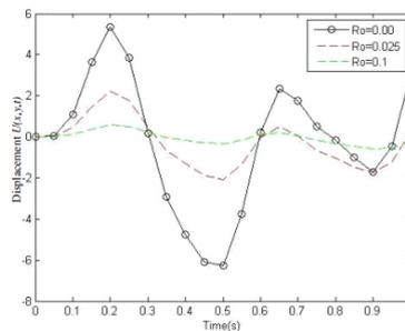
Figure 3. Effect of Rotary Inertia on Moving Force
