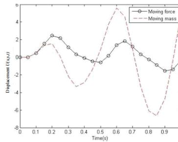
Figure 1. Moving Force vs Moving Mass
