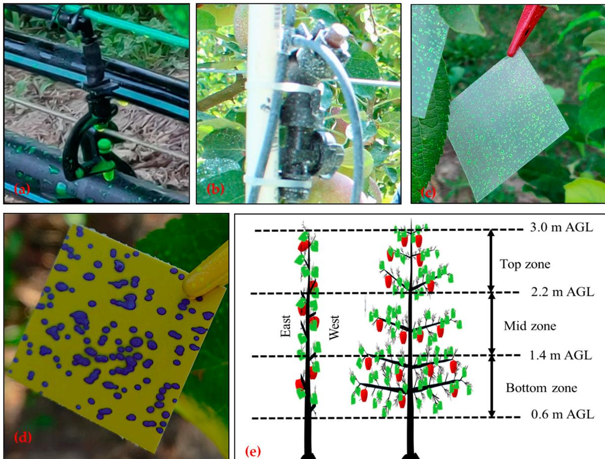
**Figure 4.** The field installation of (a) modified irrigation micro-emitter and (b) off-the-shelf nozzle utilized for respective SSCDS treatments, and the deposition and coverage analysis of the tested treatments with help of the (c) mylar card and the (d) water sensitive paper samplers installed in (e) three canopy zones on east and west side (top-east, top-west, mid-east, mid-west, bottom-east, and bottom-west).
