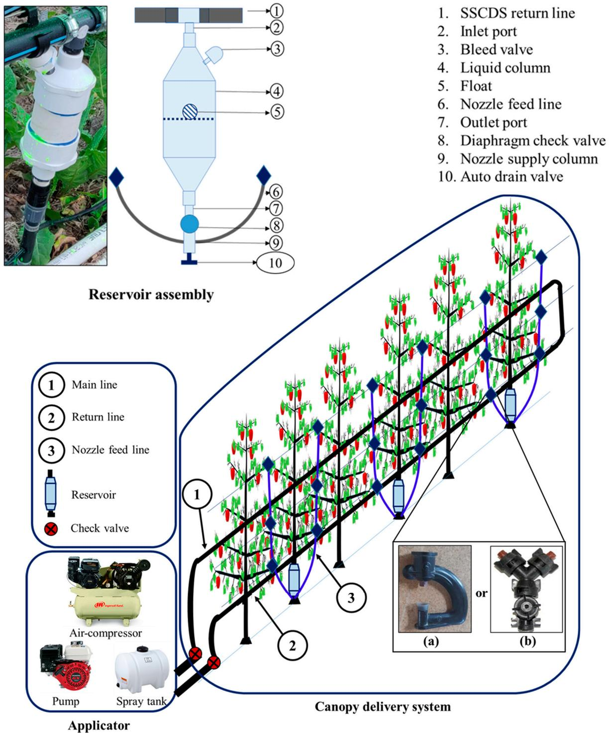
**Figure 2.** The schematics of tested pneumatic spray delivery based SSCDS with an applicator and canopy delivery system configured with (a) modified irrigation micro-emitter or (b) hollow cone nozzle in 3-tier arrangement (diamond shape with solid blue fill represents micro-emitter/nozzle).
