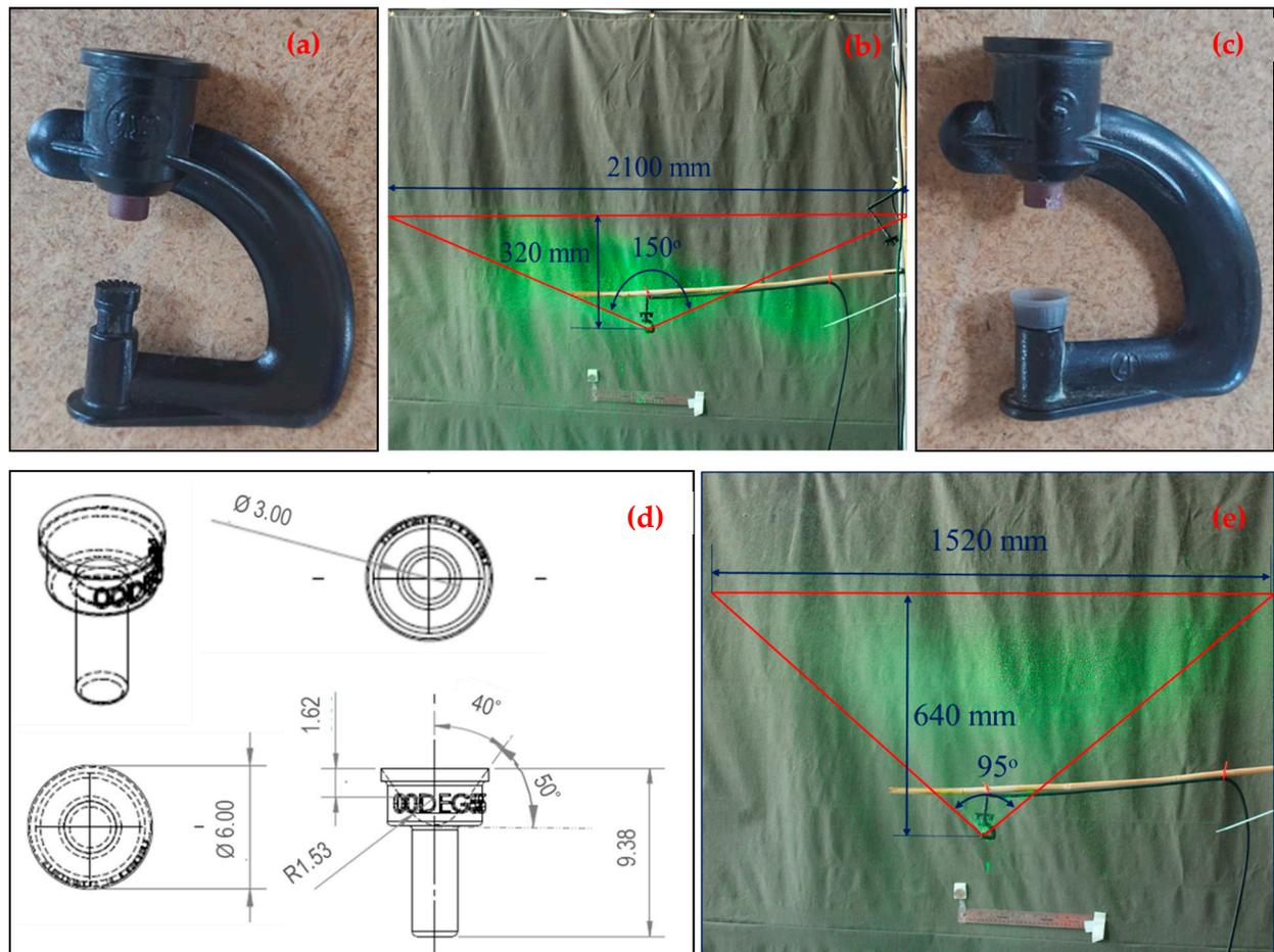
**Figure 1.** An off-the-shelf (a) micro-emitter with (b) a larger cone angle and wetted diameter, and a marginal vertical throw customized to (c) modified irrigation micro-emitter with (d) impactor plate concavity of  $50^\circ$  to acquire (e) a smaller cone angle and wetted diameter, and a higher vertical throw (not drawn to scale; all linear dimensions are in mm).
